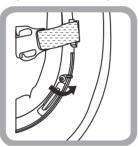
**LOCKED Position :** Safety Latch extended out over the edge of the eye protector.
