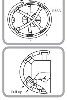
a. Remove rear four (4) cradle ribbon tabs from liner rim.
