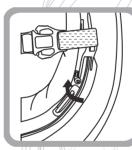
**UNLOCKED** Position : The Safety Latch rotates away toward the inside of the helmet. The Easi-on-off boss and Easi glide
